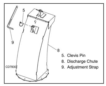
Figure 8. Discharge Chute Position
